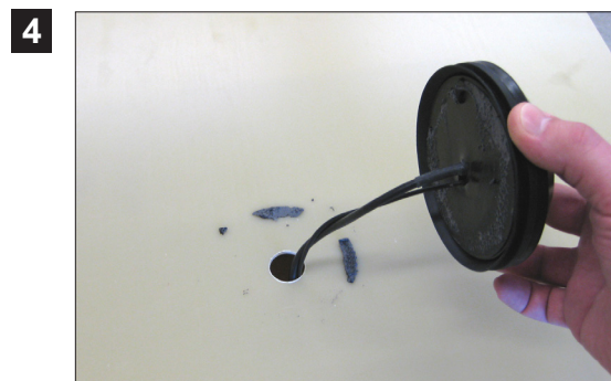
After cutting through the adhesive pad, remove the antenna and disconnect it from the wire harness.
