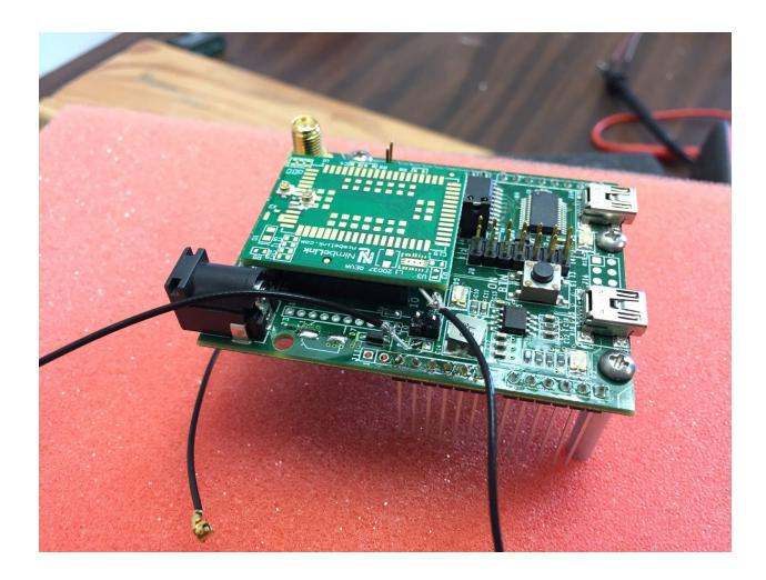
Two coax connections to the VNA are soldered to the output of the regulator on the development kit, and the input to the DC/DC on the Skywire modem. Once again, I am using a blank PCB for the Skywire modem to measure just the impedance of the traces and the pins.
