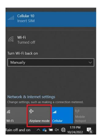
Attempt to reconnect by clicking 'Airplane mode' on and off. This should allow the modem to make a connection with Windows. Remember to turn WiFi off when testing connectivity.
