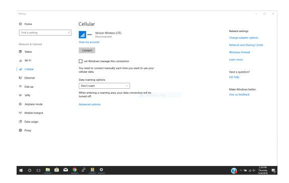
If an option for a cellular connection appears in this menu, proceed to the next section. Otherwise, make sure that the latest drivers are installed for the modem, and retry the connection.
