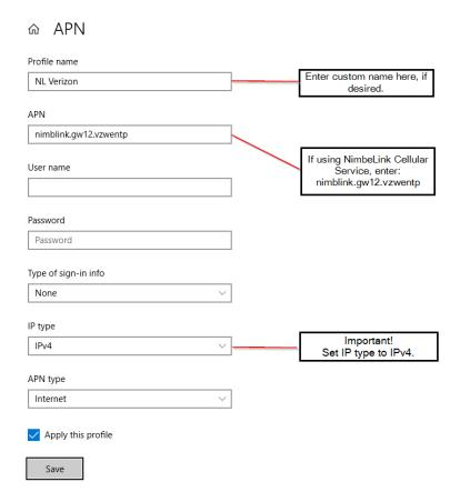
**Note:** The value of the APN field may vary. Please make sure that the APN entered into the Windows settings is the correct APN associated with the data plan being used.
