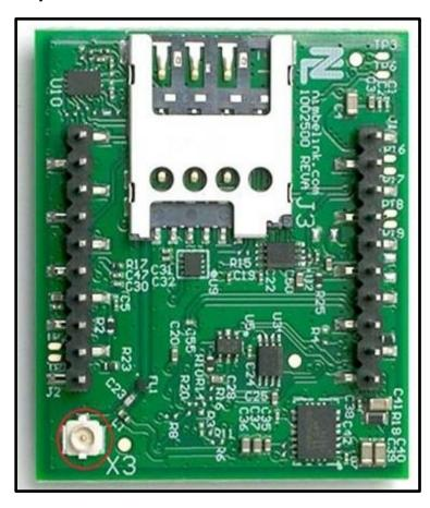
**Note:** A U.FL connector must be used when attaching the GPS antenna to X3.
