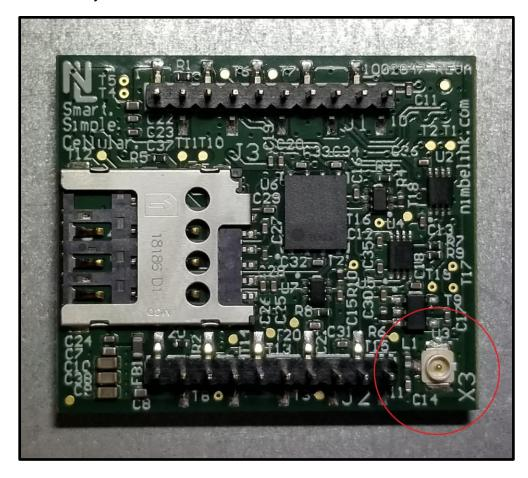
**Note:** A U.FL connector must be used when attaching the GPS antenna to X3.
