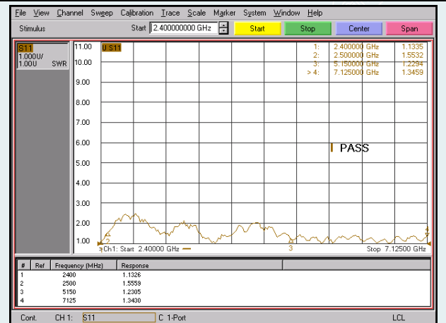
Fig.7-8 Function check after test 19# (WIFI-1)
