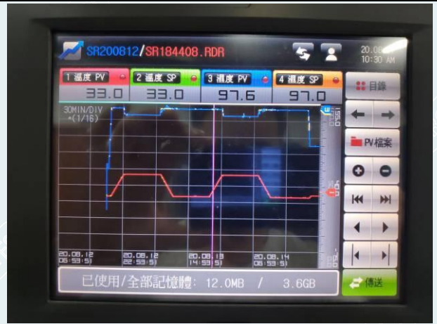
Fig.3-4 Alternating damp heat curve
