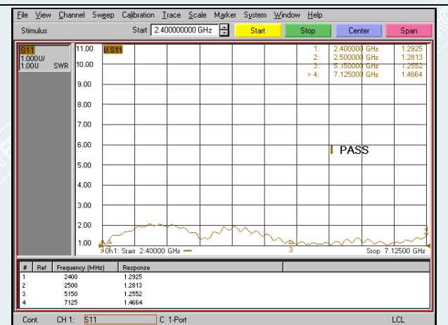
Fig.4-10 Function check after test 10# (WIFI-1)
