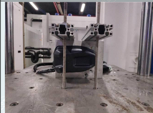
Fig.2-13 Sample installation (+Y axis 6#)
