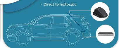
Conventional antenna + conventional internal modem 23 dBm - 2 dBm (cable loss) = 21 dBm
