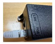
Next, connect your computer, laptop, or Wi-Fi router to the LAN port on the PoE injector.
