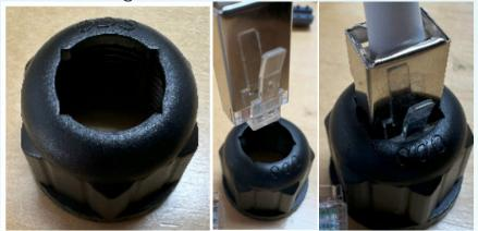
Next, insert the cable through the cable strain relief cage (D) as shown here:
