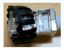
Next, assemble the 2-piece rubber water seal as shown in (C) above onto the cable. Then insert the cable through the bulkhead coupler (B). The final assembly should look like this:
