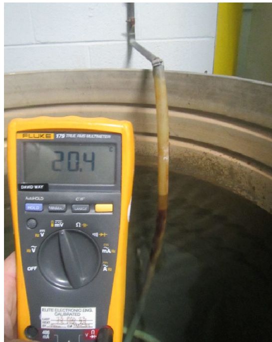
Test Setup Photograph (Water Temperature)
