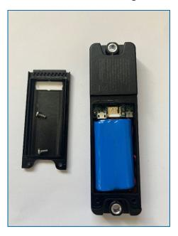
3. Using a shim, as in the video, carefully disconnect the old battery connection and discard the battery.
