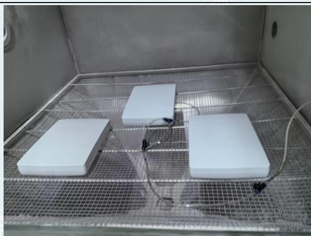
Fig.1-15 Dust proof test setup
