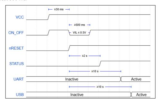
When the modem's UART interface is ready (Active) for AT commands the interface will output a 'RDY' URC.
