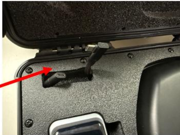
Figure 7 – Location of the power cable that connects the battery to the AC-Fleet.
