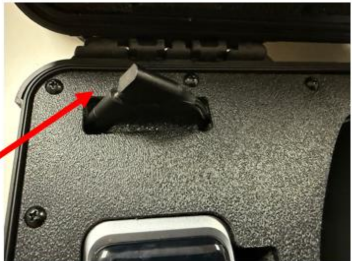
Figure 10 – Connecting the cables to turn the AC-Fleet on.
